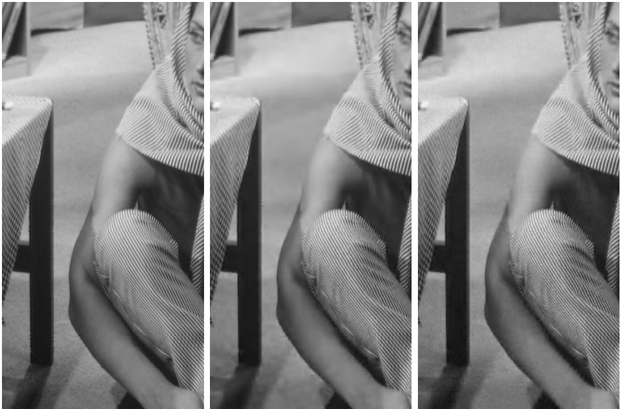
Fig.7. Example (crop) of the component based image compression for the image barbara . Left: Original image. Center: JPEG2000 compression. Right: Component based image compression. The compression ratio for both compressions is set to 0.8bpp.
