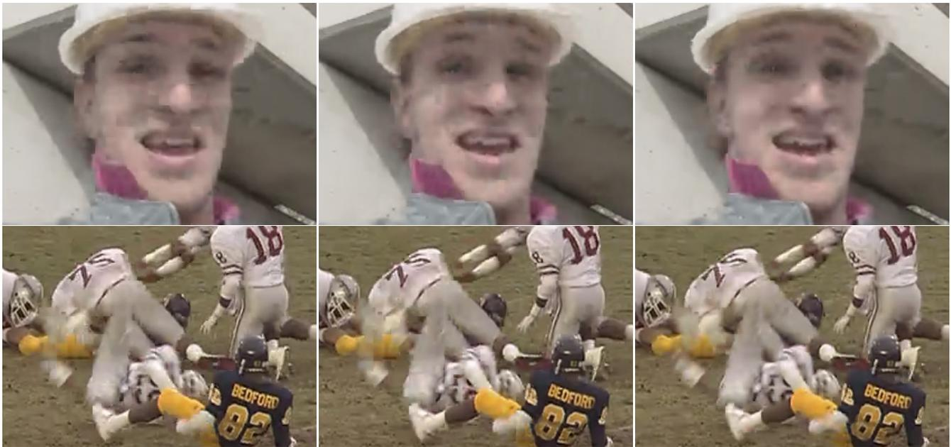
**Fig. 3.** Visual quality comparison of standard AVC encoding (left),  $(\alpha, \beta, c_0)$  optimization applying  $M_{All}$  (middle), and  $(\alpha, \beta, c_0)$  optimization applying  $M_{Canny}$  (right). All results are given for *Foreman* QP40, frame 141, and *Football*, frame 227, where details were enlarged.
