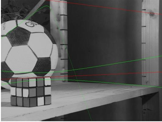
**Fig. 2.** *High insecurity for points in the background:* In this figure the effect of choosing points only in the foreground is demonstrated. We see that the insecurity for points in the background is much higher than for points in the foreground, as the epipolar band is much more extended. INRIA Syntim owns the copyright of the image.
