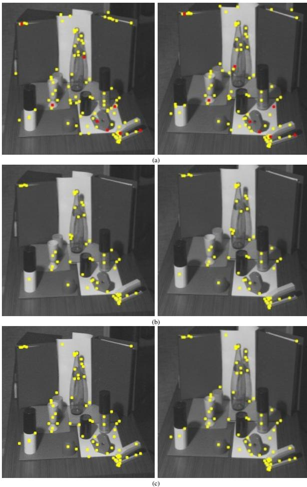
**Fig. 8.** Results: (a) stereo image pair with SIFT correspondences, the 8 points selected by RANSAC are red. (b) remaining point correspondences after outlier removal using the distance from the epipolar line. (c) enhanced point correspondence set using the new criterion. INRIA Syntim owns the copyright of the image pair.
